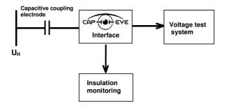
CapEye allows interconnection and simultaneous use of a voltage test system and an insulation monitoring system on one capacitive coupling electrode. The CapEye interface branches the signals to the relevant devices connected and ensures that they do not interfere with each other. In this case, it is of no significance whether CapEye forms one unit with a device or is implemented separately.
